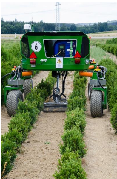
Fig. 1 Field robot BoniRob and App-Concept for mechanical weed regulation:
